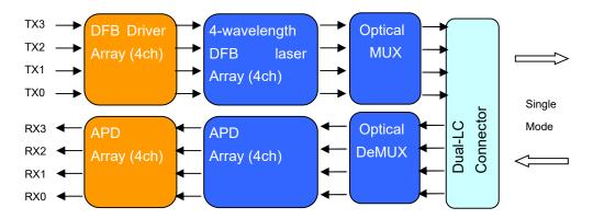
Figure 1: 40Gb/s QSFP ER4 Transceiver Block Diagram
